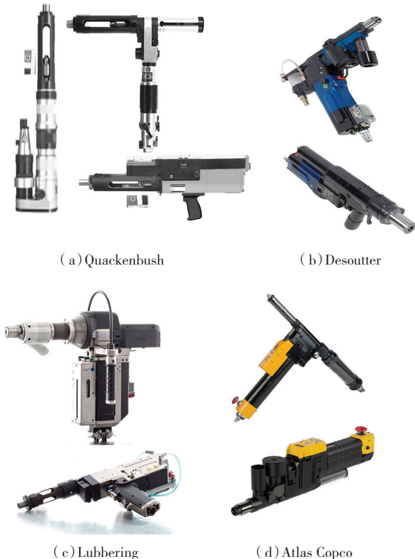
图5 典型的自动进给钻 Fig.5 Typical automatic drill unit
